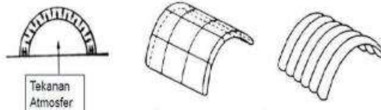
Figure 3. Air Inflated Structure
