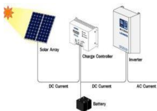
Figure 2: Photovoltaic Solar Energy Systems Source: Widayana, 2012
