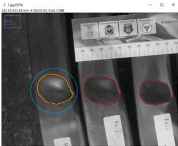
Gambar 23 Identifikasi area surface defect
