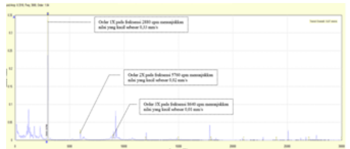
Figure 7. Pump vibration spectrum (alignment)
