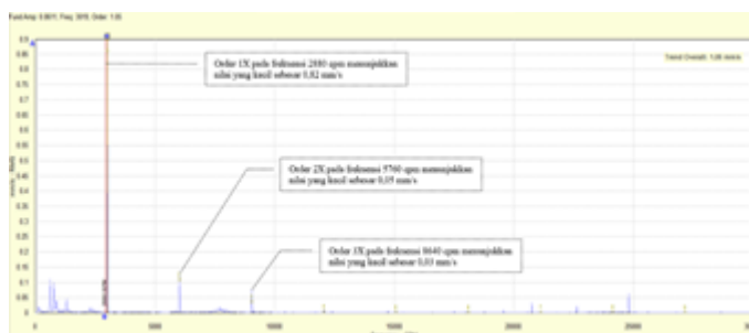
Figure 5. Motor vibration spectrum (alignment)
