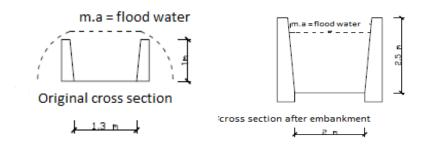
**Figure 4.** Original cross section **Figure 5.** The condition of the cross section after being given the embankment Source: Personal documents
