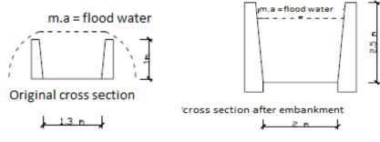
**Figure 8.** Original cross section **Figure 9.** The condition of the cross section after normalization
