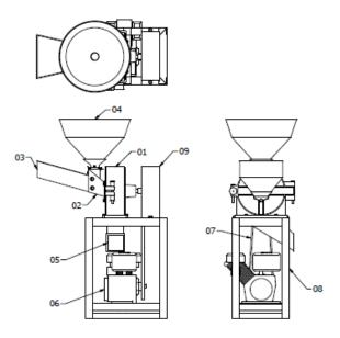
Figure 2. New Design of Disk Mill Machine
